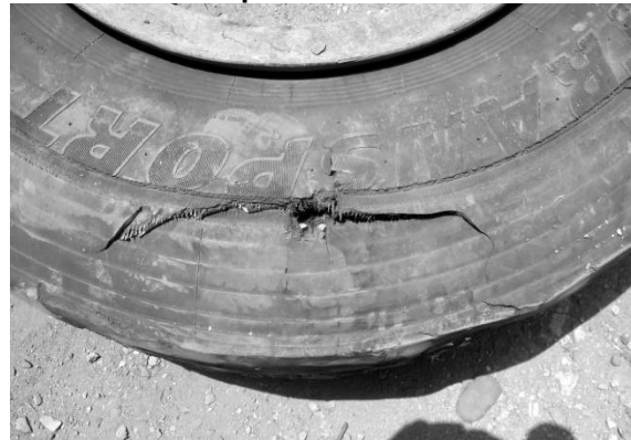
Fig. 3: Deteriorated Side Wall of the Tyre resulted in an Explosion
