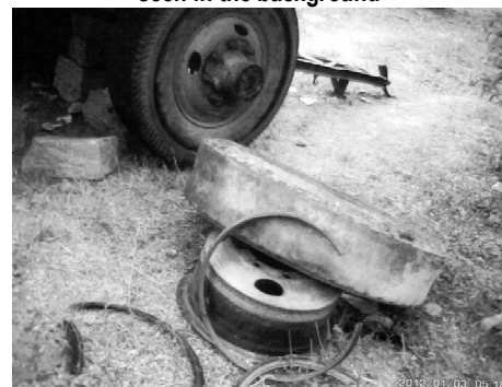
Fig. 5: Illustration showing the breaking of outer rim into 3 fragments (m1, m2 & m3), and the inner rim into 2 fragments (m4 & m5).
