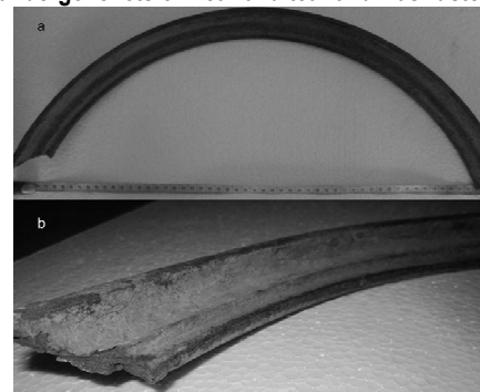
Fig. 6: (a) A fragment of the broken outer rim (m1) that was produced before us for examination. Its outer diameter measured 58 cm and weighed 1.8 kg. (b) The rim had undergone lots of wear and tear and was rusted.
